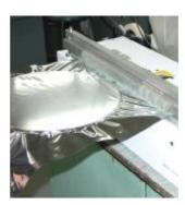
**Vacuum-Sealer, external extracting type** is used in normal packing and more in vacuum sealing, extracting air from the package or charging inert gases into the package. It has wide application, particularly suitable for packaging goods in big size, or with low vacuum and purer gas charging requirement.
