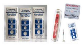
Warmmark indicator, with this temperature indicator, a proprietary red dye is released onto a blotter to clearly indicate when your shipment is exposed to temperature levels above your predetermined level, creating a permanent and immediate indication of the duration of exposure. Activation of the device is simple — remove the tab and barrier film and apply to a dry surface on your product or packaging.
