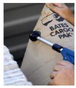
Air Blow Gun is made of stain steel and plastic material, working as an accessory tool of dunnage bag for air inflation. It works with air compressor by connecting the nozzle with the tube. It can also be used to dedust machines, equipments, instruments, apparatus etc.
