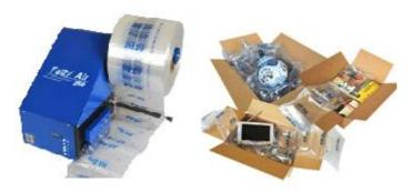
Fatty Air Cushion Packaging System is an efficient, safe and economical solution of protection packaging. It forms air bags, which is inflated with air and used to fill the cartons according to your needs. This kind of package has great excellent performance of shock resistance.
