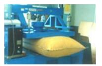
Pressure test in China Packing Research & Test Center(CPSTC) Our dunnage bag remains undamaged at the maximum of 9 tons of pressure Maximum pressure capacity: 0.2Bar/20Kpa/2.9P.S.I
