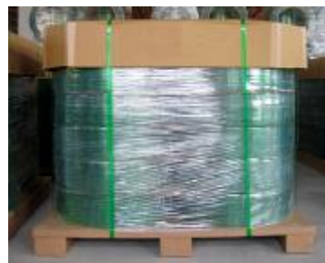
strapping of palletized goods
