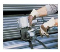
**Steel strap** is generally used in packaging heavy and big dimension goods due to its greatest strength and most durability.
