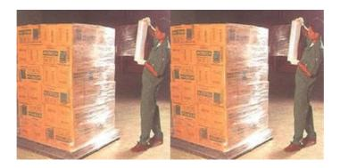
Hand Stretch film: The hand wrapper is the simplest implement for Conventional Hand-Stretch film wrapping. The film is mounted on a frame where unwinding of the film can be slowed down by turning a handle. This is to allow a certain degree of stretch control.
