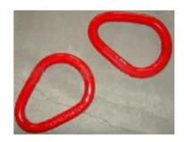
Pear shaped link is made of high quality alloy steel through swaged forging process. It's small size, light weight and high strength. Its max proof load is 2 times of rated load and min breaking load is 4 times of rated load.
