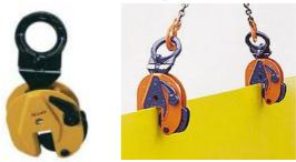
Vertical Plate Lifting Clamp is used in single or one pair for vertical lifting of steel plate. The max lifting weight of single clamp is called rated capacity. It can only lift one piece of plate each time. Multi-Plates lifting is prohibited. Collision shall be avoided during lifting. When lifting, the locking handle must be turned upward to make the spring tense. When unloading, it should be turned downward. The clamp and plate can be separated only after spring loosing.
