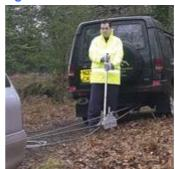
Wire Rope Pulling Hoist is a light hand lifting equipment, a combination of the hoist and wire rope. It's a general tool with multi-function of pulling, lifting, lowering, tensioning and securing spacing objects. It's widely used in rescue, transportation, logistics and other fields.
