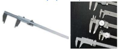
Heavy-Duty Vernier Caliper is an instrument for measuring length. It's made up of main scale and sliding nonius attached on it. The main scale's unit value is millimeter. Compared with common vernier caliper, it is stable and durable, mainly used for objects of large measuring range,.
